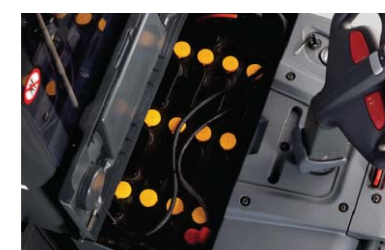
Standard battery Long operating time through high capacity with 3 PZS battery.
