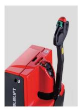
In particular through the long tiller design the operator can always keep a safe distance to the truck during proceeding the work very ergonomically. The design ensures lower operational forces than trucks with a short tiller. The tillers operating height is naturally positioned to ergonomic, operator friendly controlling positions.
