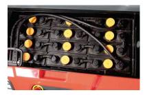
Optional sideways battery exchange compartment for PT20L with 210 Ah battery.
